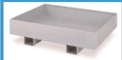
Capacity 250 litres - formed from 3mm sheet steel with fully welded seams. Ground clearance 100mm
